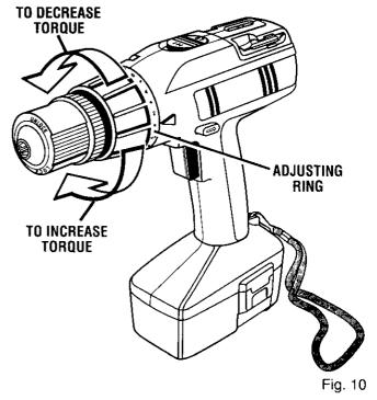
Note: Remember the two-speed feature (HI-LO) when setting torque. The amount of torque will vary depending on which speed setting you have your drill-driver. Switching to LO speed will increase torque. Switching to HI speed will decrease torque.
